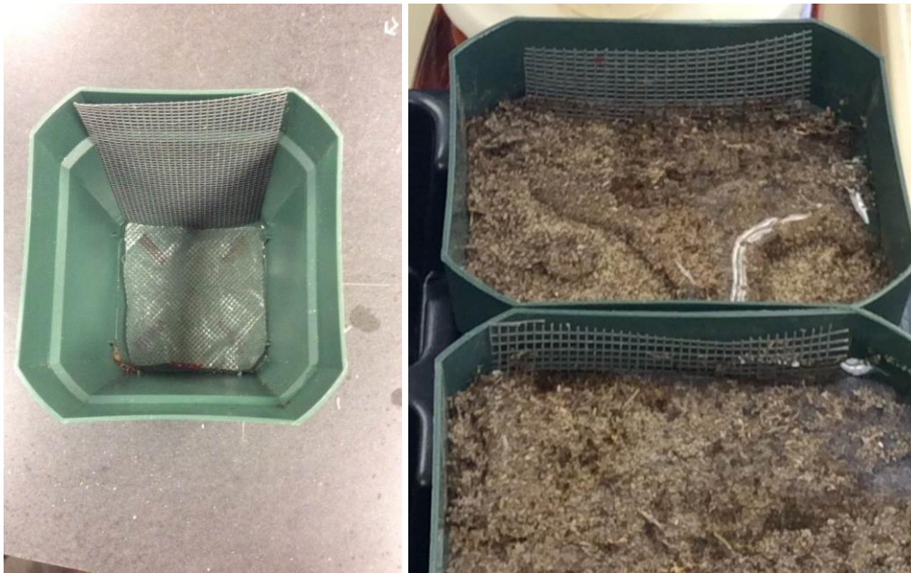
Fig. 1. Illustration of design of pots used in Pot Studies 1 and 2. Pot on left shows nylon mesh covering bottom and vertical screen on side of pot. Pots on right show pots filled with hydrophobic soil immediately after application of 40 ml (0.25 inches) of water.
